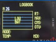
RATIO iX3M DEEP: the above first 11 dives (\*), each ca. 1 h, consumed 76 %, 100 → 24 per 19.10. [(\*) 12.10. was one SCUBA dive, but computer changed to 2 free dives ...] After the 12th. dive (09.11.), during SI: jump from 18 % battery capacity to 0 % thus #26 is on LOW BAT
