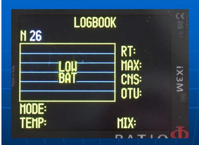
RATIO iX3M DEEP: jump from 18 % battery capacity to 0 %
