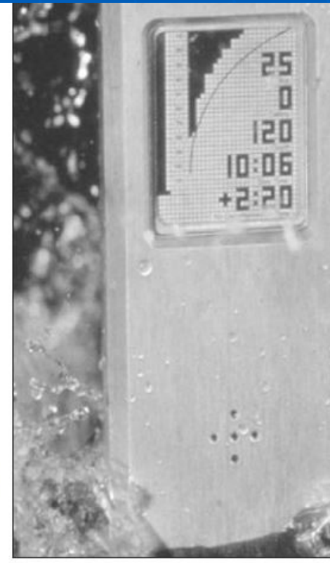
Figure 4-10. A. The Orca EDGE (Electronic Dive Guide Experience), the first commercially successful digital dive computer. The display of the EDGE had a bar graph that represented the computed nitrogen tension (in fsw) in each of 12 Haldane tissues.
