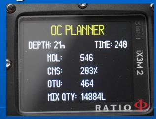
the NOAA / USN Ox-Tox implementation still questionable: for EAN 50 it should give s.th. around 290 % of a CNS ox-tox dose and OTU: 450 the NDL is, according to the EAN50 table from A. A. Bühlmann, ca. 270 min:
