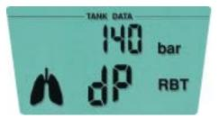
At the conclusion of a dive the Smart COM displays the "differential pressure". This value represents the gas that is consumed during the dive. Also displayed are any warnings that may have occurred throughout the dive, in this example both RBT and Workload warnings are displayed.
