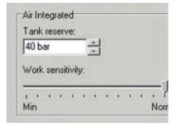
With the Smart TRAK software that is supplied with the Smart COM, the sensitivity of the workload setting can be set by the diver according to their own level of fitness.
