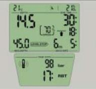
Smart TRAK replays actual screen data for the Smart COM and the Smart PRO in 4 seconds intervals.
