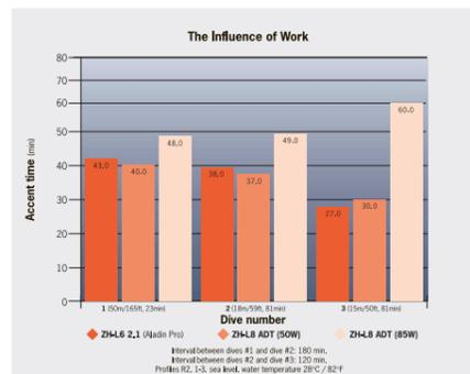
Earlier mathematical models assumed a mean workload output of 50W. With the ZH-L8 ADT MB model, even at level 0, if workload is increased to 85W then on a (15m) 50ft dive the ascent time is increased from 30 to 60 mins.
