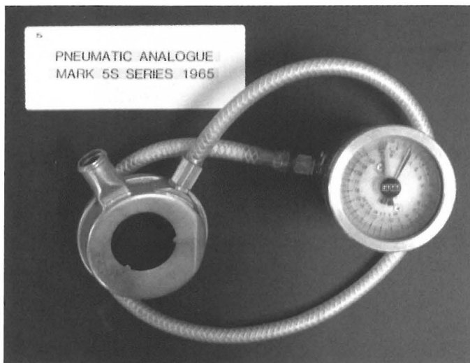
MK5-S Diver-carried computer plumbed directly into the casing of an "Aqua-Master" scuba regulator.
