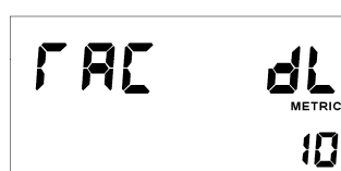
Figure 33 PROGRAMMING MODE (Setting TACITE On Time) On Time 10 sec
