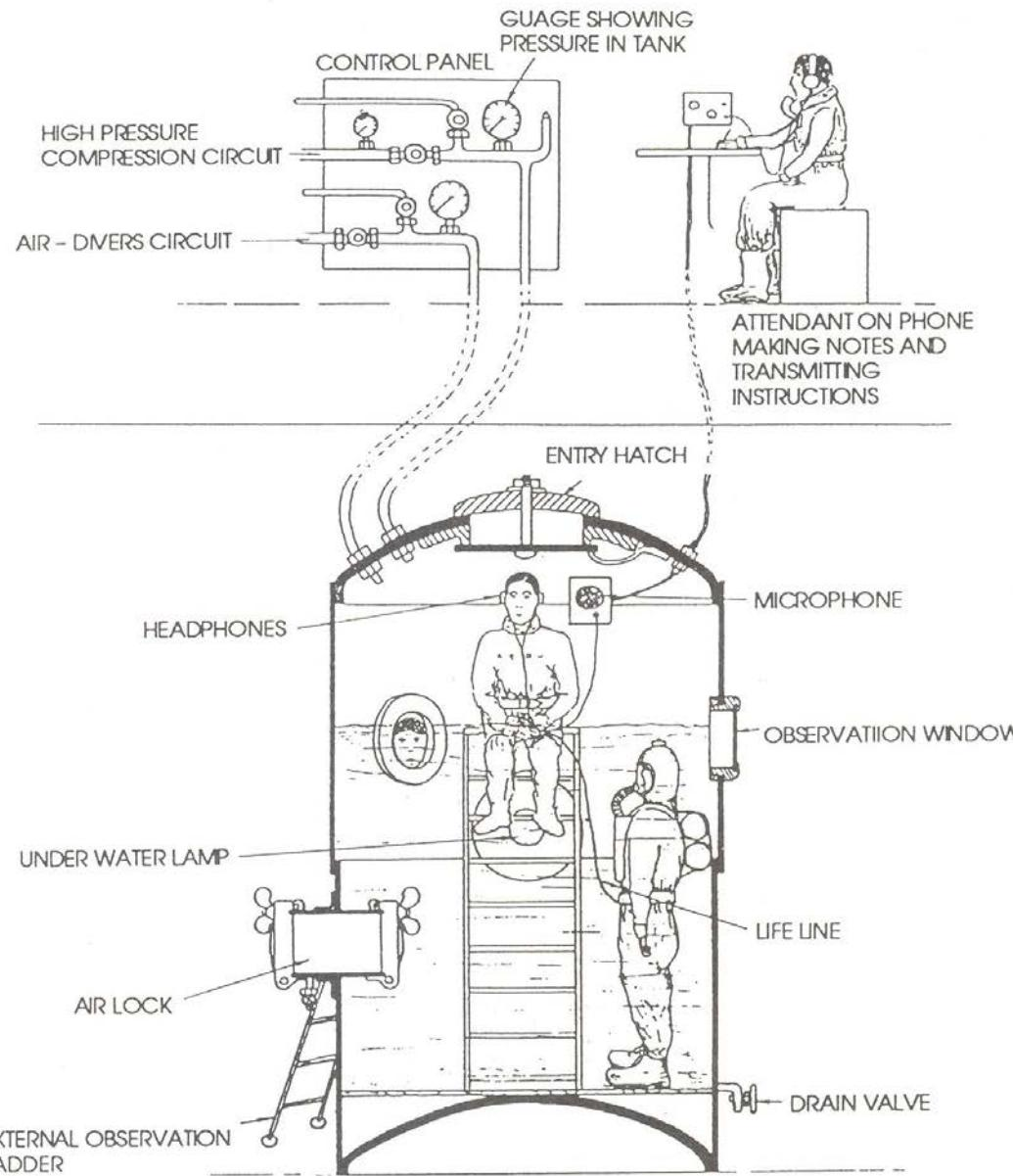
FIG. 2 Showing wet pressure chamber with diver under water breathing oxygen in self-contained set. Internal and external attendants.
