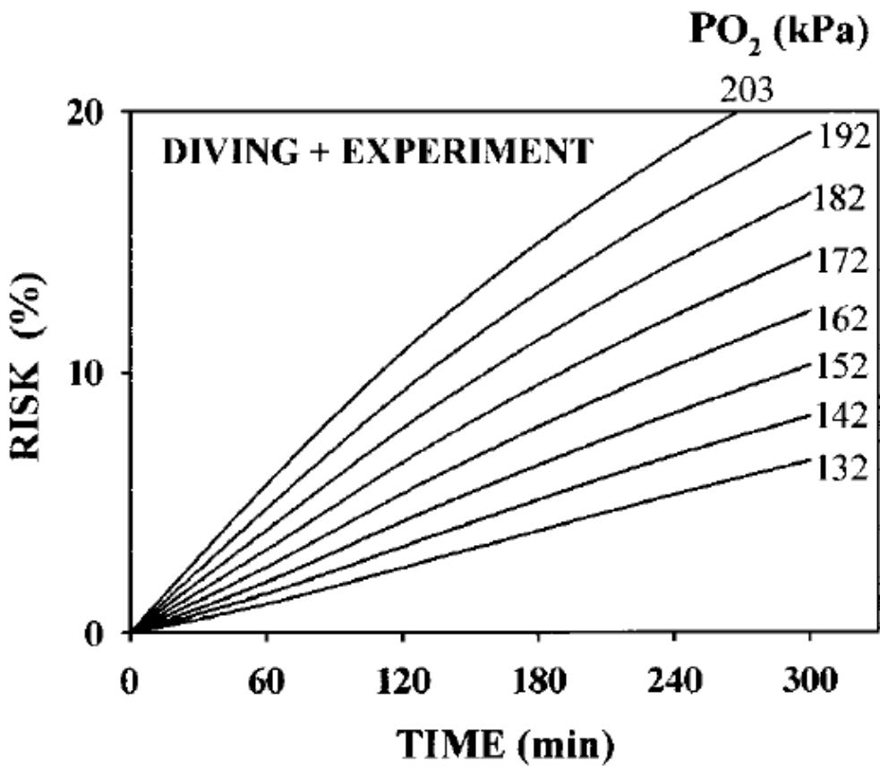
Fig. 8. Percent risk of CNS oxygen toxicity as a function of time and  $\text{PO}_2$ . The parameters for the calculation were derived from both hyperbaric experiments and diving.
